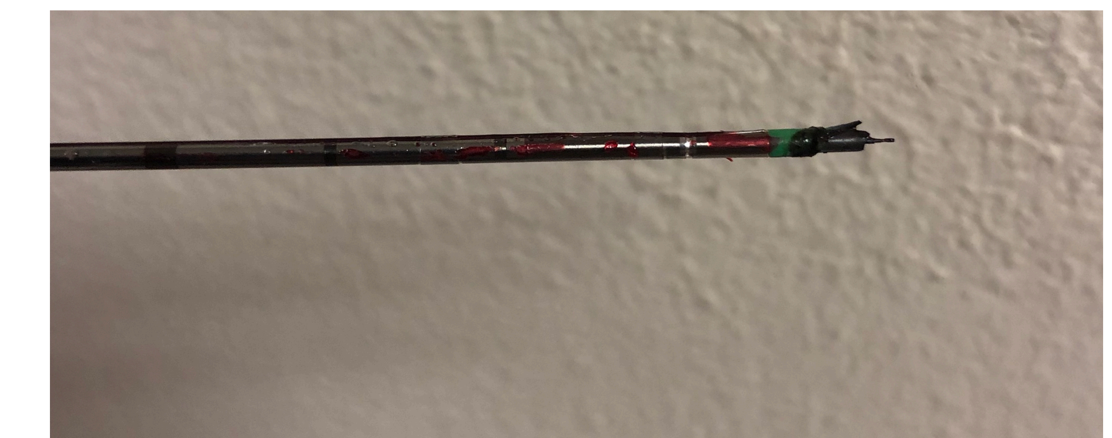
Figure 4: Photograph of fractured antenna probe at time of the procedure.
